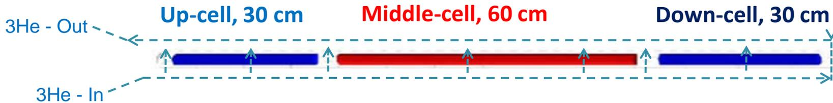
**The target consists of granulated crystalline ammonia ( $\text{NH}_3$ ) loaded in three cylindrical cells .**
