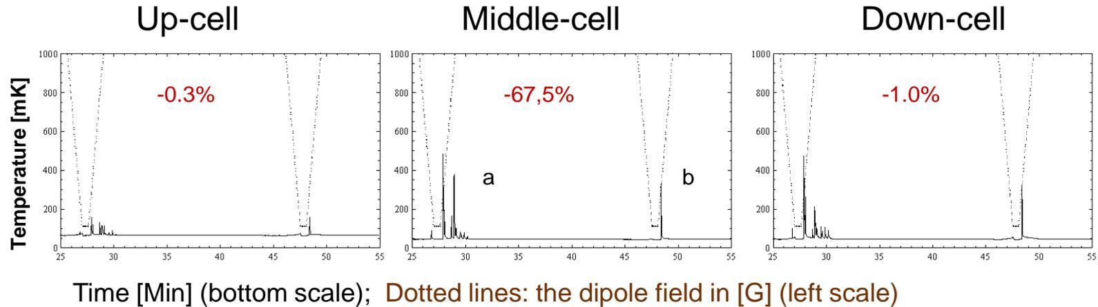
1. The change of nitrogen alignment nearby 0.03 T field excites the lattice vibratory spectra. The plot shows an nondegenerating (a) and degenerated (b) magneto-mechanical spectra of  $^{14}\text{N}$ ; the effect is absent at static field.
