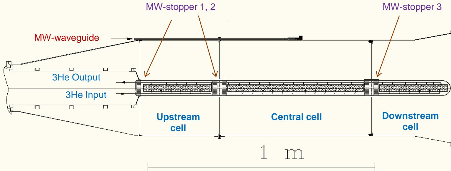
1. Target **volume** of bout:  $400+800+400 \text{ cm}^3$ , **Surface**  $\approx 1.5 \text{ m}^2$
