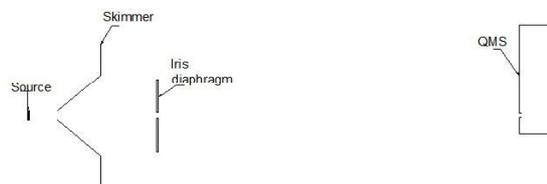
Figure 1. Schematic diagram of apparatus for measurements of radial size of a source of hydrogen atoms.
