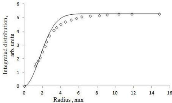
Figure 5. Integrated distribution of the hydrogen atoms source density.  $\diamond$  - experimental data for  $N_{H_2} = 5 \cdot 10^{17}$  mol/pulse. Solid curve is the fit using Gaussian radial density distribution with characteristic radius of 2.4 mm.
