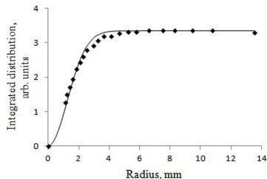
Figure 4. Integrated distribution of the hydrogen atoms source density. ◆- experimental data for  $N_{H_2} = 3 \cdot 10^{17}$  mol/pulse. Solid curve is the fit assuming Gaussian radial density distribution with characteristic radius of 1.79 mm.
