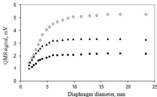
Figure 2. The QMS signal (H-atoms) vs the iris diaphragm diameter. ■ - number of hydrogen molecules injected into the dissociator tube per pulse is  $1.5 \cdot 10^{17}$  mol/pulse, ▲ -  $N_{H_2} = 3 \cdot 10^{17}$  mol/pulse, ◇ -  $N_{H_2} = 5 \cdot 10^{17}$  mol/pulse.
