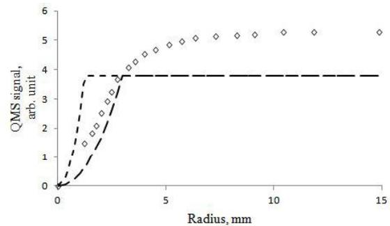
Figure 3. Comparison of the experimental data (◇ -  $N_{H_2} = 5 \cdot 10^{17}$  mol/pulse) with curves for expected QMS signal vs radius at source position. The curves show expected QMS signal for homogeneous source density distribution and for radius of the source equal to the dissociator nozzle radius - 1.25 mm (dashed line) and to the skimmer radius - 3 mm (long-dashed line).
