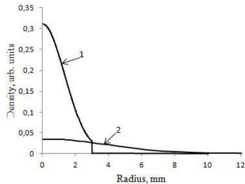
Figure 7. Radial hydrogen atoms density distribution correspondent to the two - Gaussian fit shown in Figure 6. The experimental data were fitted by sum of two Gaussian curves. Curve (1) was cut at the skimmer radius (3 mm).
