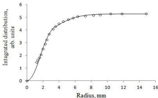
Figure 6. Integrated radial distribution of the hydrogen atoms density.  $\diamond$  - experimental data for  $N_{H_2} = 5 \cdot 10^{17}$  mol/pulse. Solid curve – fit assuming two-Gaussian radial density distribution with characteristic radiuses of  $R_1 = 1.9$  mm,  $R_2 = 4.2$  mm.
