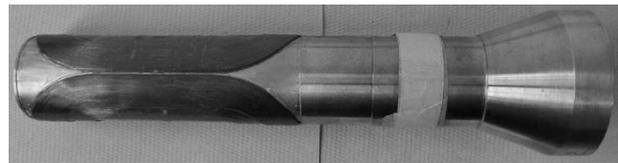
Figure 5. The internal superconducting holding coils for transverse field operating at 1.2 K can be seen.
