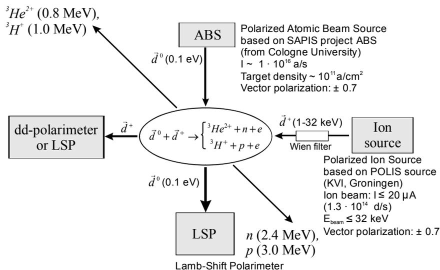
Figure 2. Layout of the experiment.
